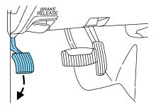
The BRAKE warning lamp in the instrument cluster illuminates and remains illuminated (when the ignition is turned ON) until the parking brake is released.
